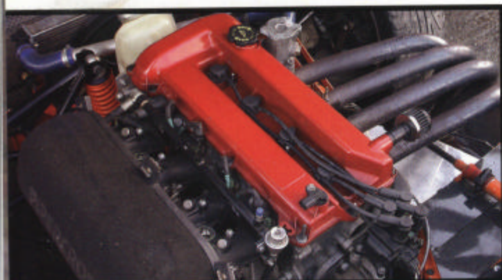
Raceline tuned 2-litre Ford Duratec produces 225bhp.
