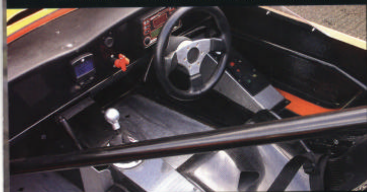
To save weight, doors are bolted to the body so you have to hop over them to gain access to the sparsely equipped cockpit.
