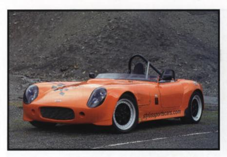
side deflectors are more basically handled, but the effect is nonetheless striking. A serious triangulated rollbar leaves you in no doubt of this car's intentions, with bare carbon seat shells, full harnesses and a stripped-out interior equally blatant. A weight saving exercise means the doors are bolted into place and lack any hinges, so it's hop over the top and slide down into position. An aftermarket Tillett carbon racing seat isn't especially comfortable and the SSC seat shell on the
